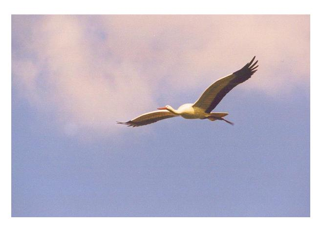
Believe it or not you're looking at an electric RC model of a stork. It was built in Germany using a complex geodesic internal framework. The motor is up front and a long drive shaft extends to the rear propeller. That prop folds back during glide to become the storks' legs which normally trail behind in flight just as you see in the picture.
